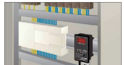
Example of DIN rail mounting in control panel
