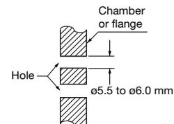
2. Mount the optical joint part to the vacuum chamber wall. When mounting to the vacuum chamber wall, the O-ring included with this product must be attached and the side to which it is attached must be the atmospheric side.
