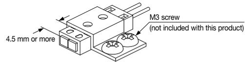
If mounting using an M3 set screw (cup point)
