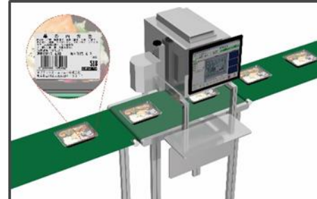
Inspection of use-by dates printed on packages
