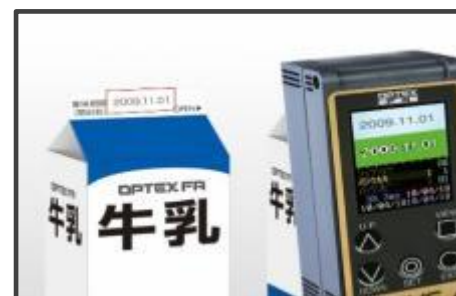
Inspection of use-by dates printed on milk cartons
