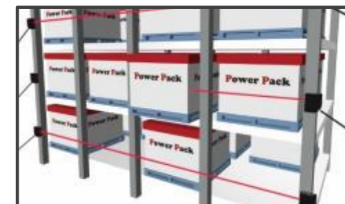
Detecting boxes protruding from shelves in automatic warehouses
